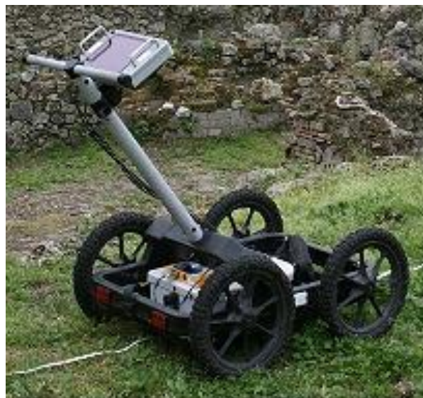
Figure 6. A GSSI GPR system mounted on a four wheeled cart.
