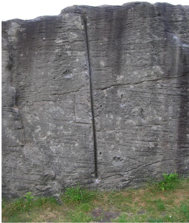
Figure 13. Part of a large block of millstone grit in Padley Gorge waiting to be split into smaller blocks.
