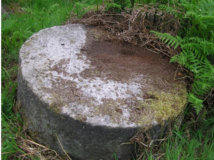
Figure 13 A shaped cylindrical stone before its central hole had been cut. Padley Gorge. (Author's photograph)
