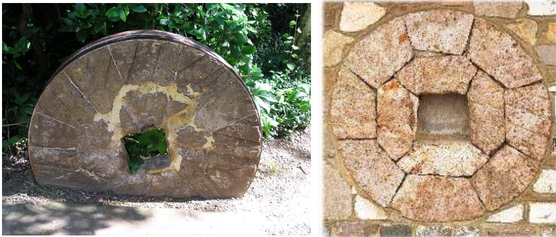
Figure 11. Used French burrstone from Lode Mill on the left and a new one on the right. (Author's photograph)
